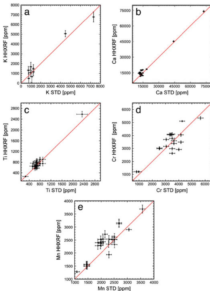
**Figure 5.** Handheld X-ray fluorescence (HHXRF) measurements on meteorite samples plotted versus reference (STD) values obtained by ICP-MS and XRF. (a) K, (b) Ca, (c) Ti, (d) Cr, (e) Mn, (f) Fe, (g) Co, (h) Ni, (i) Sr and (j) Ba. The red line shows 1:1 linear correlation. Note the logarithmic scale in the Ba, Ni and Sr plots.
