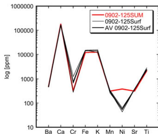
**Figure 7.** Handheld X-ray fluorescence measurements of soil samples from the find site of meteorite RaS 316 (field No. 0902–125) in Oman. Sample SUM refers to 'soil under meteorite' and shows a strong enrichment of Ni as compared with measurements of reference soil samples from the surface (Surf).
