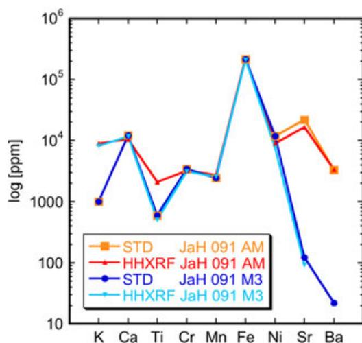
**Figure 3.** Data for two samples (median values of 4 HHXRF measurements) of Ba-spiked and Sr-spiked standard pressed pellets compared with expected values (STD). In the high Ba sample JaH 091 AM, the Ti content is overestimated because of overlapping of Ti  $K\alpha$  and Ba  $L\alpha$  lines. Note the elevated K values observed in the pressed pellets produced with sodium silicate (water glass).
