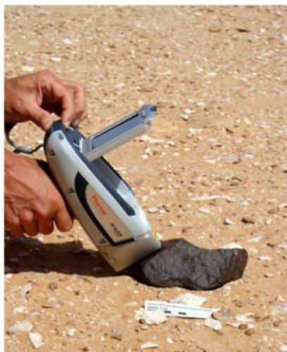
**Figure 2.** *In situ* handheld X-ray fluorescence analysis of a meteorite (RaS 309) discovered in the desert of Oman. Note the high contrast between the dark meteorite and the light colored soil.
