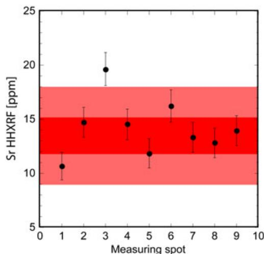
**Figure 4.** Strontium variation in a large cut slab of the Allende CV3 meteorite. All data points represent measurements of 300 s. Dark red: all available reference values<sup>[30]</sup> (Actlab 2009 & 2010); light red: corresponding error box. Sr is not homogeneously distributed in meteorites. Therefore, we recommend using weighted mean values.
