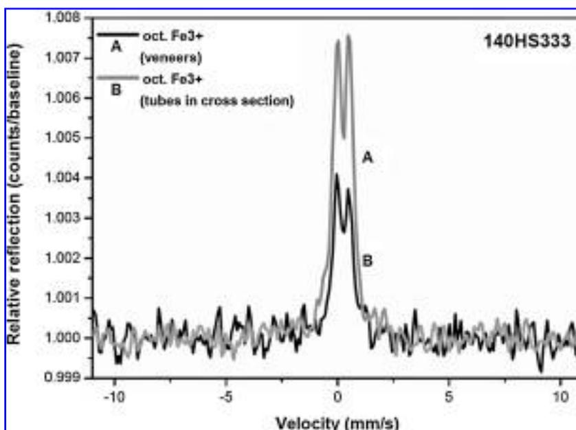
FIG. 12. *In situ* Mössbauer spectra of sample 140HS333 (freshwater limestone, Ries Crater, Germany) showing difference in iron content between dolomite veneers (A) and exposed tube surfaces (B). Instrumentation: Beagle 2 QM Mössbauer Spectrometer. Data courtesy University of Mainz, Germany.
