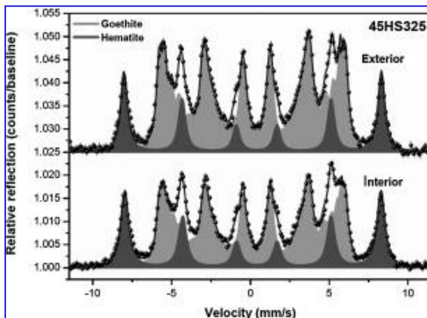
FIG. 15. *In situ* Mössbauer spectra of sample 45HS325 (Fe-encrusted filaments in chalcodony vein, Cady Mountains, USA). Two iron phases are present, hematite and goethite. Goethite is more pronounced on external (more yellow) surfaces. Instrumentation: Beagle 2 QM Mössbauer Spectrometer. Data courtesy University of Mainz, Germany.
