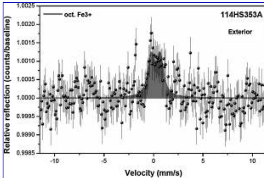
FIG. 19. *In situ* Mössbauer spectrum of sample 114HS353A (orthoquartzite, McMurdo Dry Valleys, Antarctica). The weak signal associated with external “oxidized” surfaces is due to iron being present as very thin grain coatings. Instrumentation: Beagle 2 QM Mössbauer Spectrometer. Data courtesy of University of Mainz, Germany.
